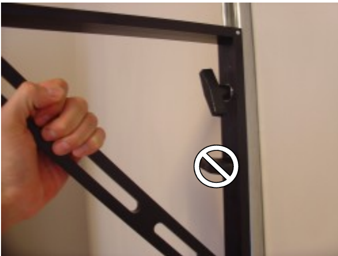
Left: Sliding the bracket up the track. Note: This is a smaller (shorter height) track. We now use the larger track for more strength.
